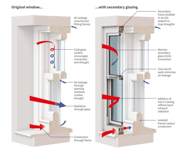
The secondary window traps an insulating mass of air between the inner and outer glass and the resulting warmer surface of the inner glass limits convection currents. Isolated frames are also less conductive and draughts are significantly reduced by efficient seals applied both to the frame and opening panels. If a low-E coating is applied to the inner glass, it will reflect back infrared radiation and so retain energy in the room.
