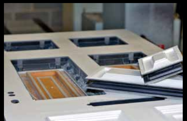
Door after routing operation
