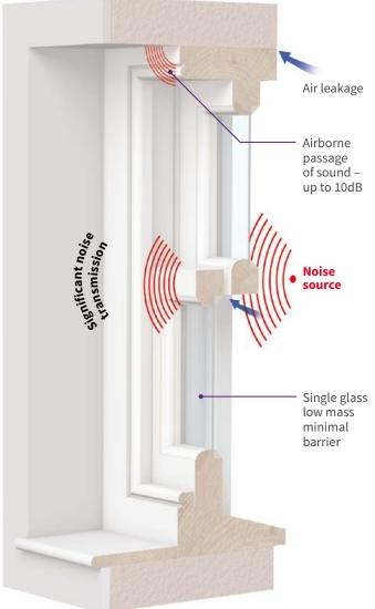
Air leakage Air leakage Larger cavity 'decouples' the windows and reduces noise
